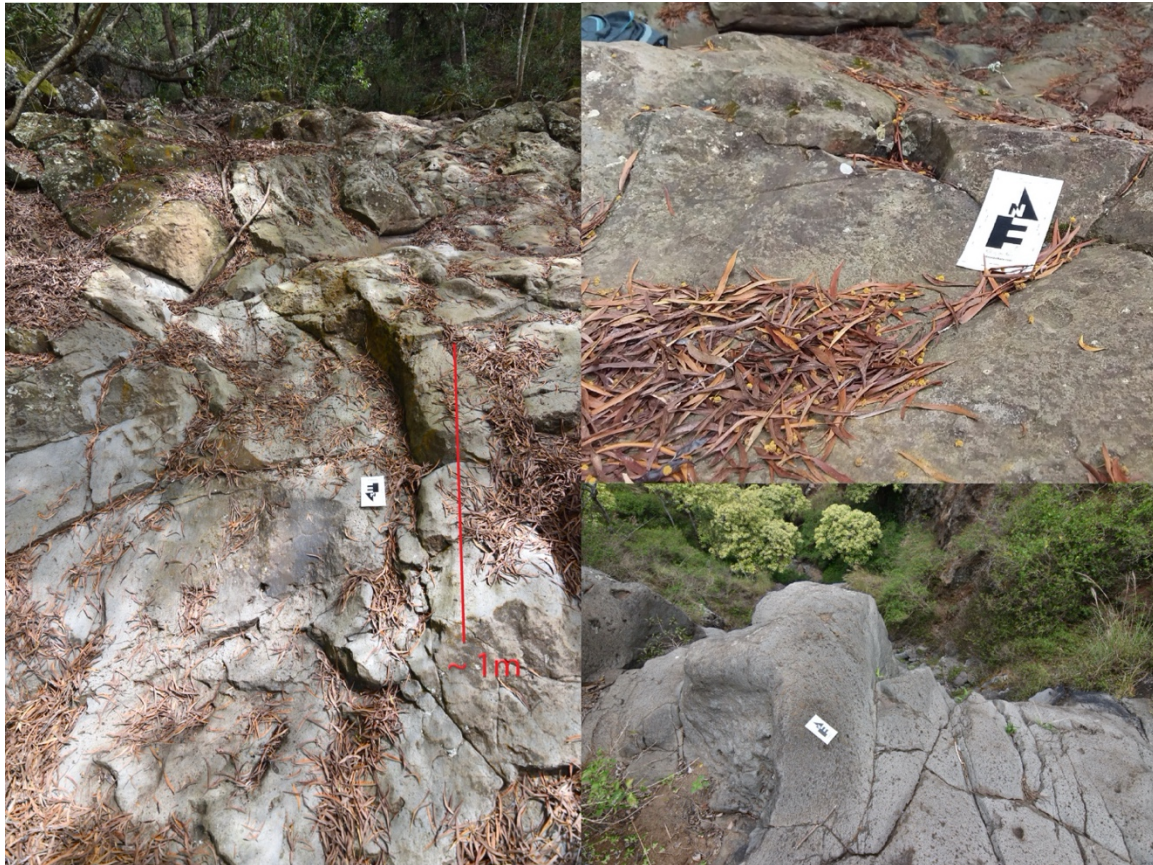
Figure A1. Photos of bedrock conditions at or near the lips of waterfalls. Scale in photos is 10 cm. In virtually all case it was impossible to confirm joints were through going and in general joint width varied considerably and most blocks appeared firmly attached.
