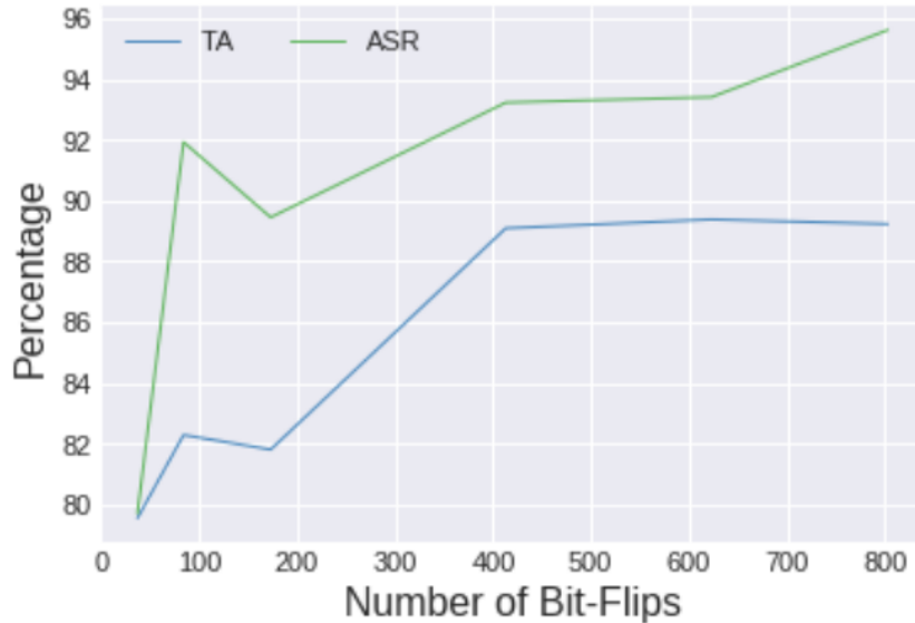
Figure 3.4: ASR (Green) And TA (Blue) vs Number of Bit Flips Plot. Only with 84 Bit Flips TBT Can Achieve 92 % Attack Success Rate (7).
