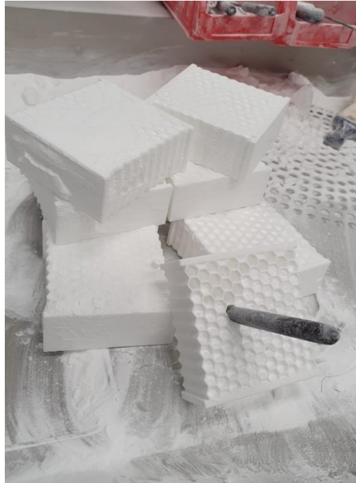
Figure 33: Post-processing of honeycomb specimens
