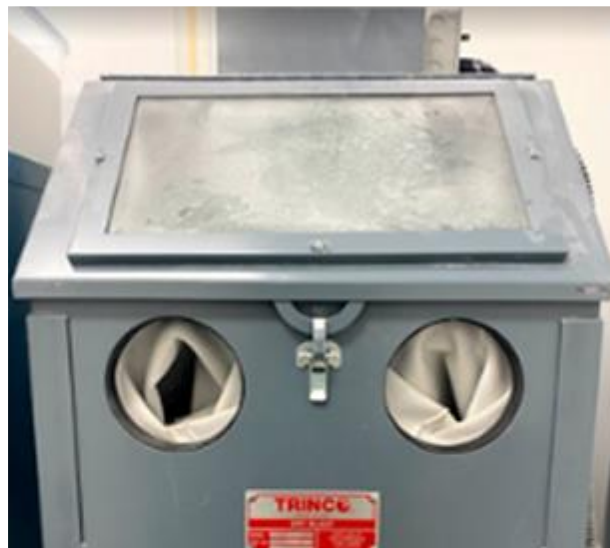
Figure 34: Bead blasting of the specimen with glass powder
