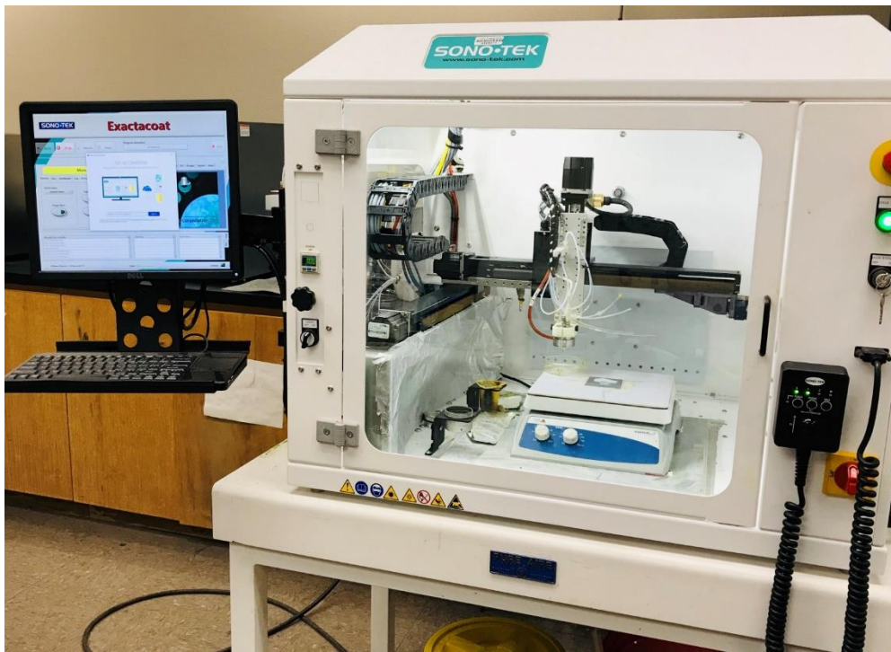
Figure 7 Ultrasonic spray coating machine for thin-film fabrication
