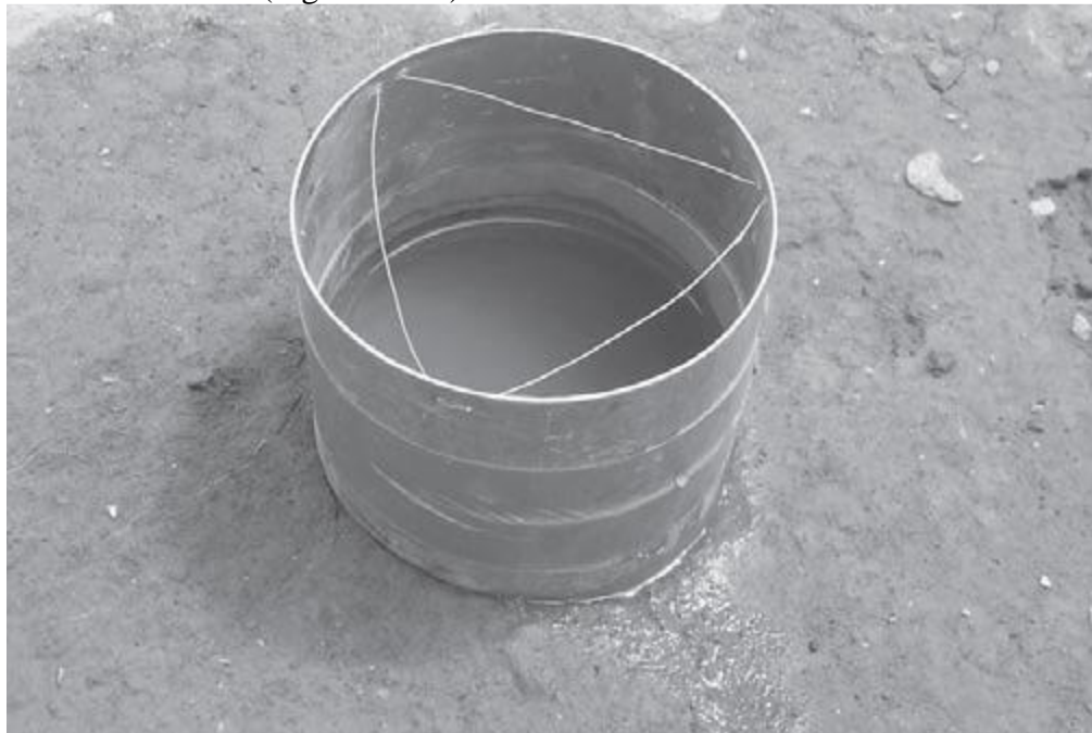
Figure K.4.6. Water leaking from the infiltrometer ring.
