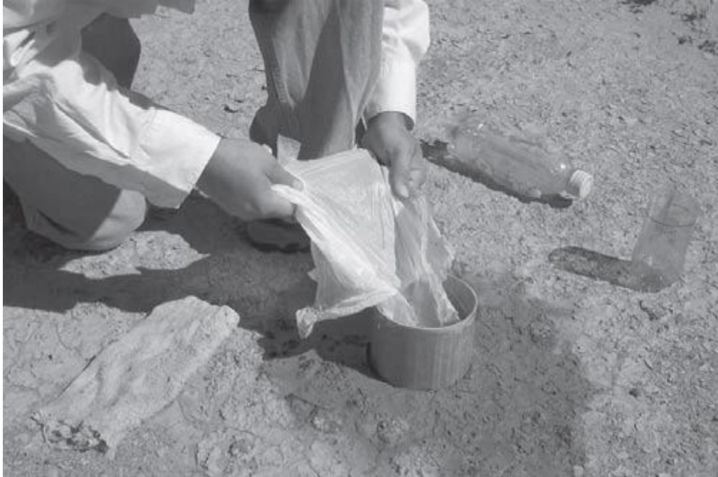
Figure K.4.5. Adding water to the ring using a plastic bag.
