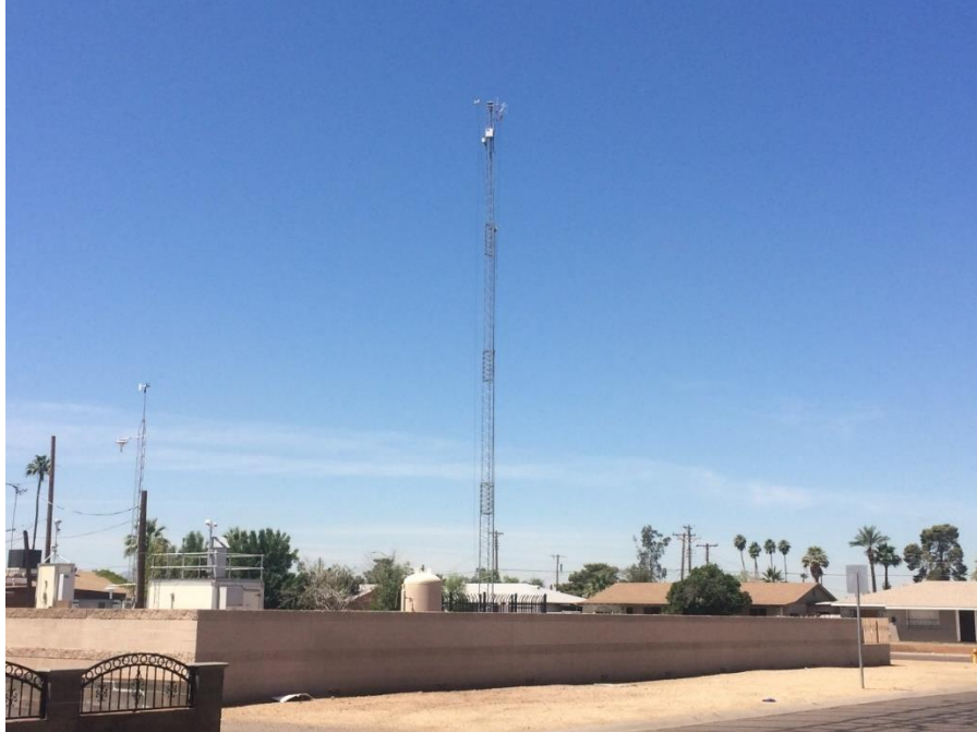
Figure L.1.4. Eddy covariance tower of the Suburban Reference site. Credit: Nicole Templeton.
