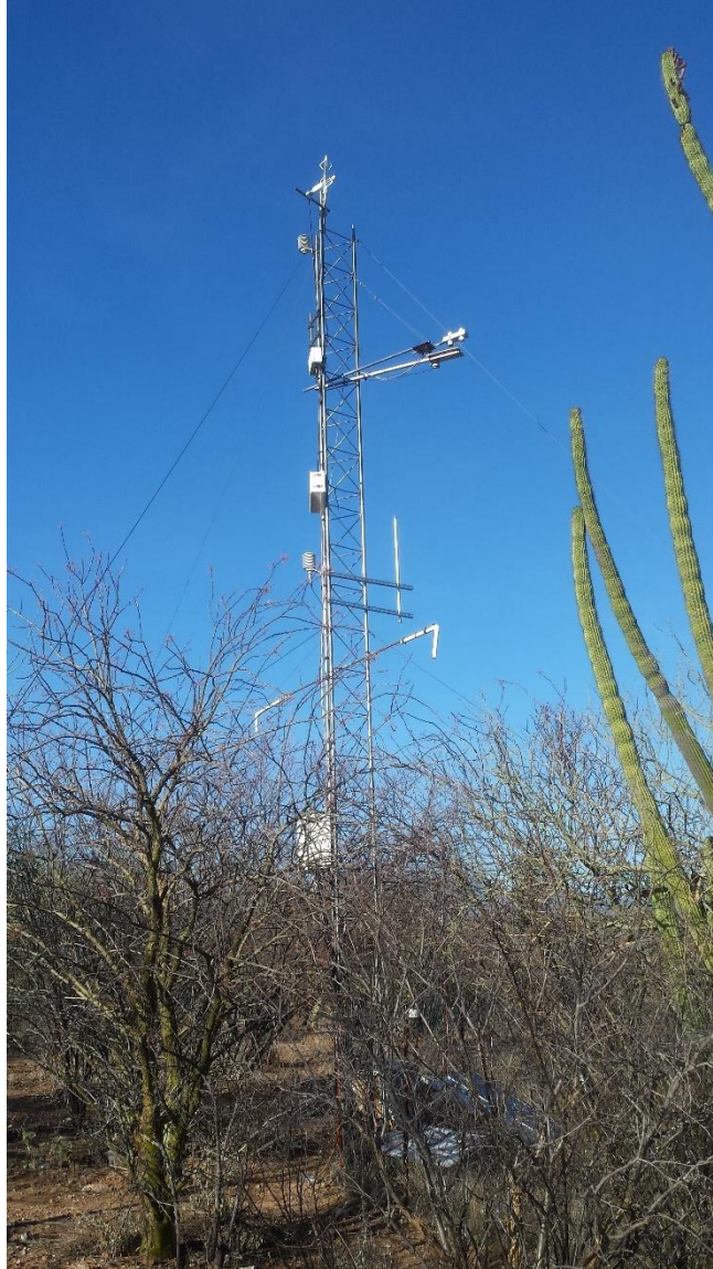
Figure L.2.1. Eddy covariance tower in the Subtropical Scrubland site.
