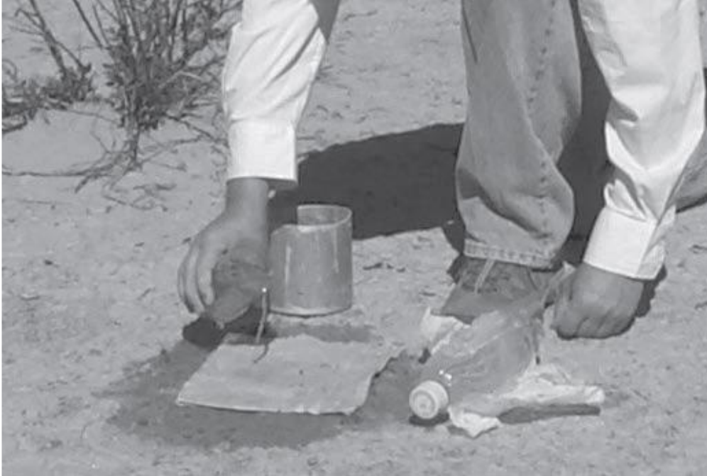
Figure K.4.3. Pre-wetting of the soil.
