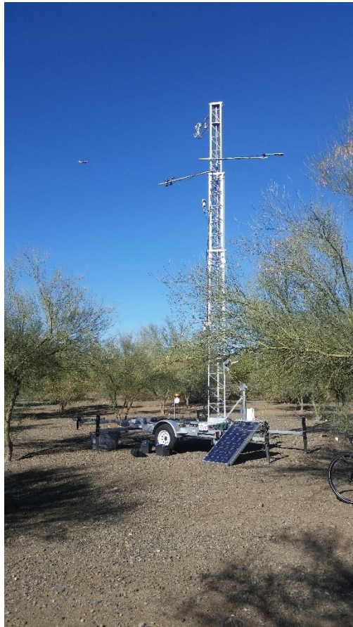
Figure L.1.1. Eddy covariance tower installed in the Xeric Landscape. Credit: Nicole Templeton.
