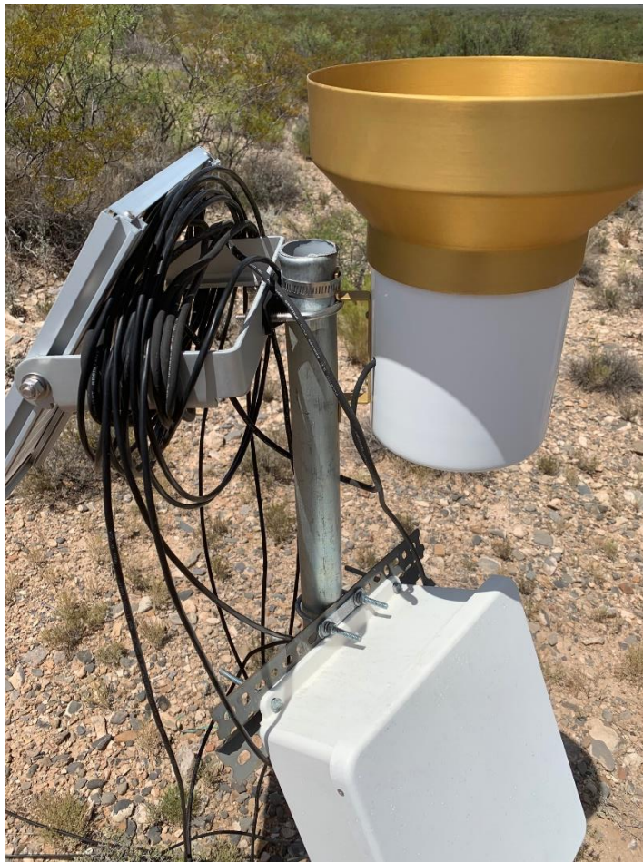
Figure L.3.21. Rain gauge and datalogger case in one of the soil moisture transects in the Tromble Weir watershed. (Credit: Zachary Keller).
