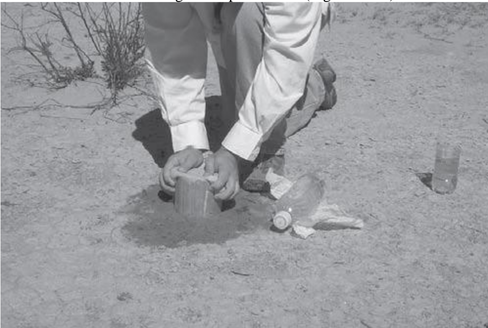
Figure K.4.4. Inserting infiltration ring to 3 cm.
