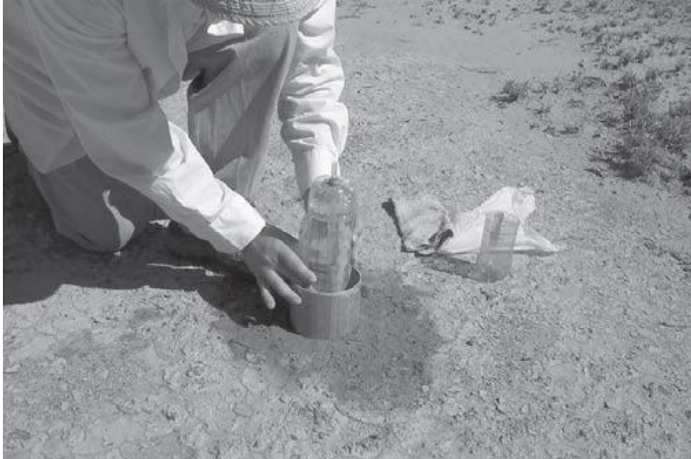
Figure K.4.7. Suspending the infiltrometer water bottle in the infiltrometer ring.
