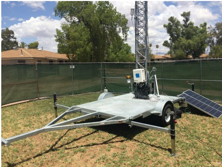
Figure L.1.5. Photograph of the mobile tower used to setup the eddy covariance system.
