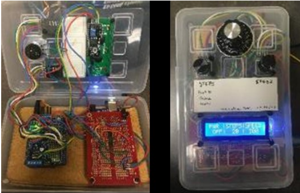
Figure B.1: Project Box containing Actuator Controller and FSR integration
