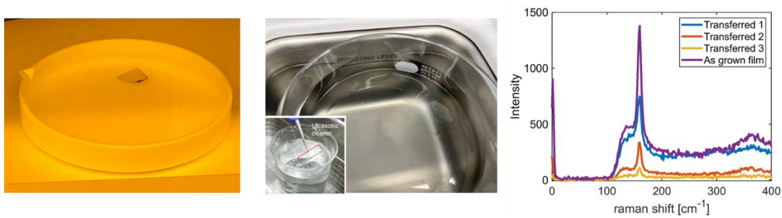
Figure 31. (a) Bi 2 O 2 Se film on Mica merged in 16% HF solution (b) A bubble math sonication peel off the film from Mica and allow transfer on to Si substrate (c) Raman spectra shows films quality consistency after wet transfer
