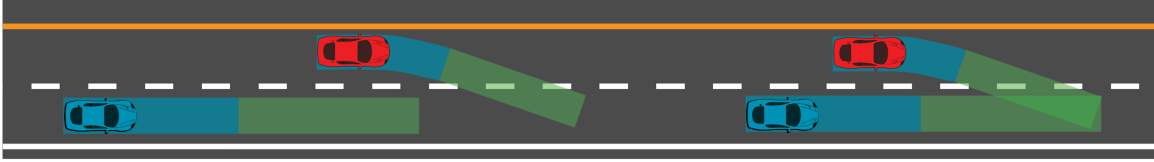
Figure 3.1: Vehicles are in safe state, if their REs (green shade) do not overlap (left) or if the REs overlap, but CEs do not overlap (right). This is because both vehicles can avoid the accident by proper braking.
