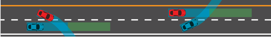
Figure 3.2: Two vehicles are in a crash state, if the CEs of two vehicles overlap. The accident may be un-avoidable. In the left figure the blue vehicle has the ROW, while in the right figure the red one has ROW.
