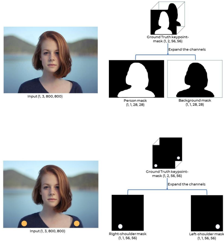
Figure 2.4: Mask R-CNN Class-wise Output Feature Map (Top) and Keypoint Encoding in Output Mask (Bottom) (Image courtesy: Patil (2021))
