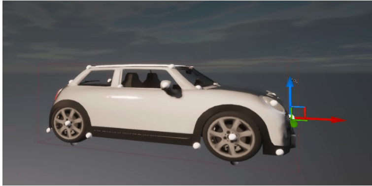
Figure 3.4: Mini Cooper Annotations. White Spheres on the Vehicle Are 3d Annotation Points.
