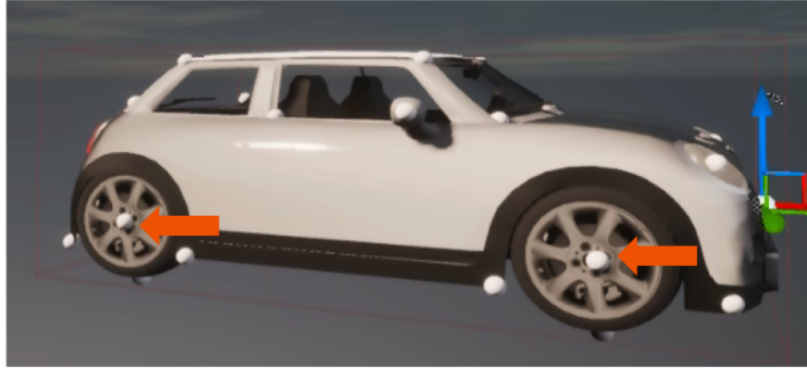
Figure 3.2: Annotated 3d Model of Carla's Mini Cooper Vehicle, Red Arrows Pointing to the Wheel Centers.
