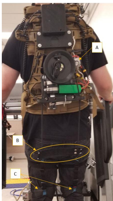
Figure 19 Post-updated A-LCPS with a View of Cross-strap and Incremental Encoder Attachment to Motor.
