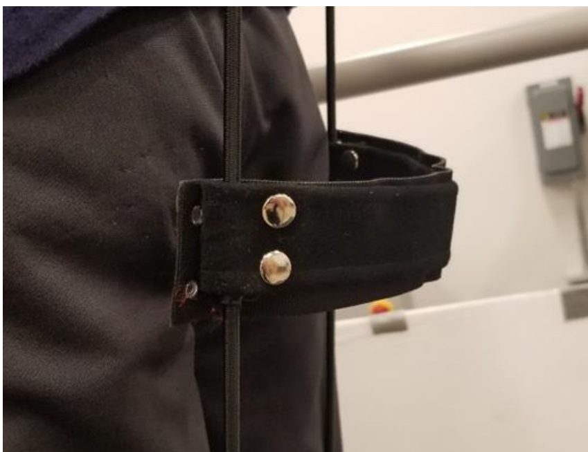
Figure 8 Bungee Cross Strap Support, Preventing Separation of the Bungees below the Bungee Guide and above the Knee Attachment.
