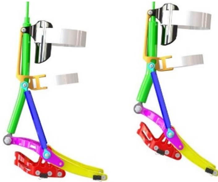
Figure 42 Comparison of Actuated and Non-actuated Prototype States. A – Non-actuated State of the AAFO, B – Actuated State of the AAFO.
