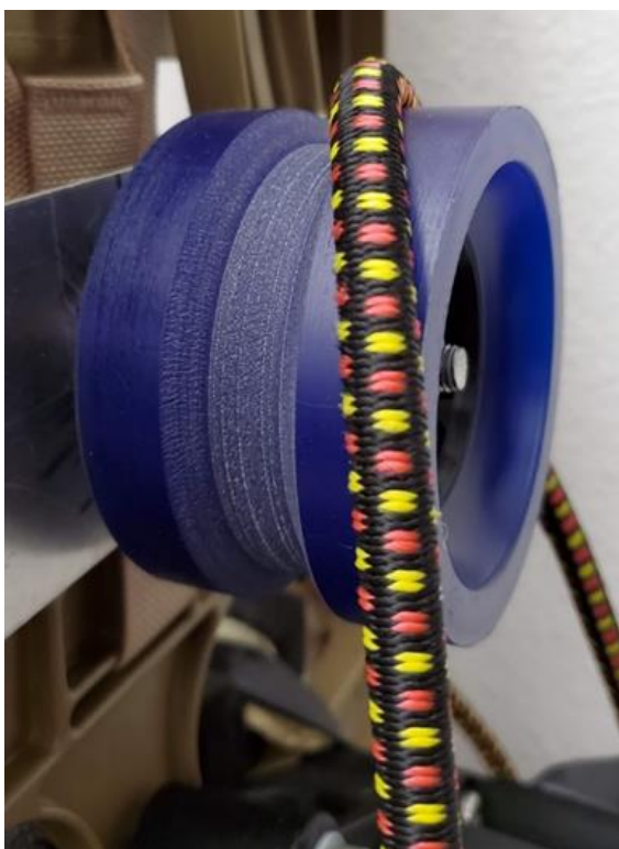
Figure 7 Pulley Made from a Modified Longboard Wheel.
