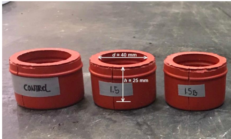
Figure 3-5. Silicon mold used for asphalt binder samples production and testing (“h” corresponds to the inner depth of the mold).
