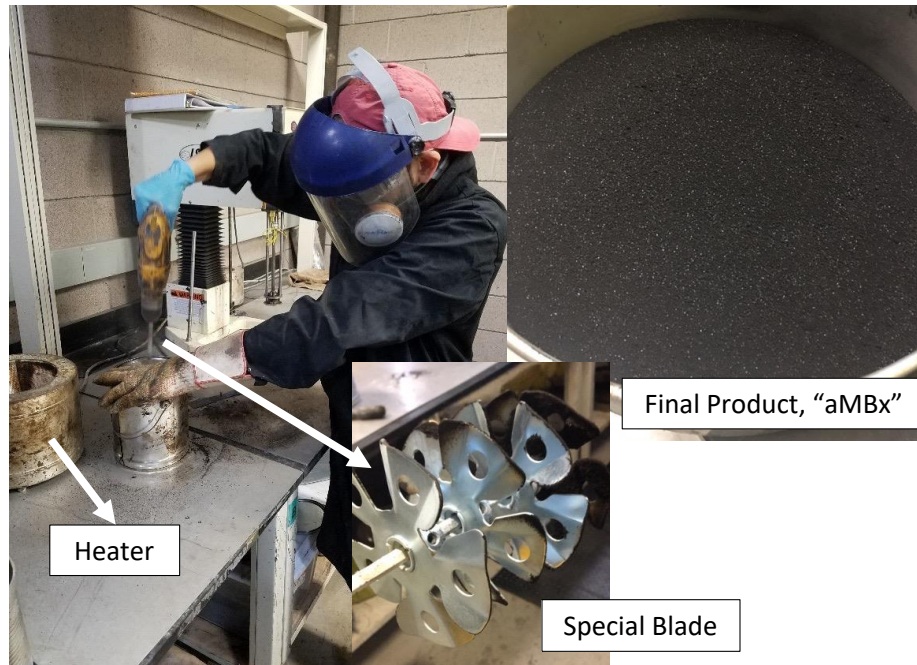
Figure 5-3. Manufacturing of aMBx.
