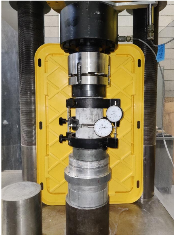
Figure 5: 3.2.2.1 Testing machine and setup according to ASTM C469 to calculate modulus of elasticity.
