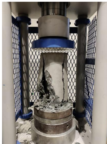
Figure 3: 3.2.1.2 Compression testing machine with cylindrical specimen failed in compression.
