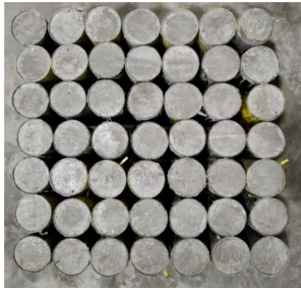
Figure 2:3.2.1.1 Cylindrical specimens casted to obtain the mechanical properties of the concrete mix.
