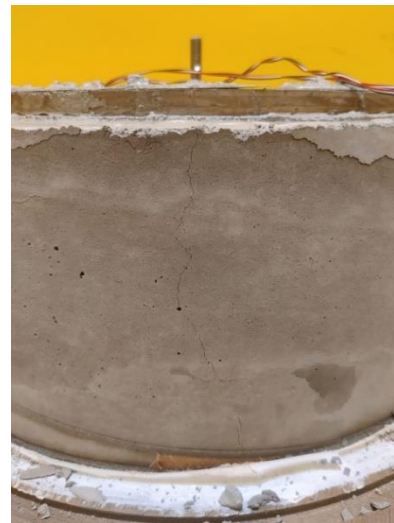
Figure 18: 4.3.2 Strain data from all four sensors along with the crack for the CPC mixture.
