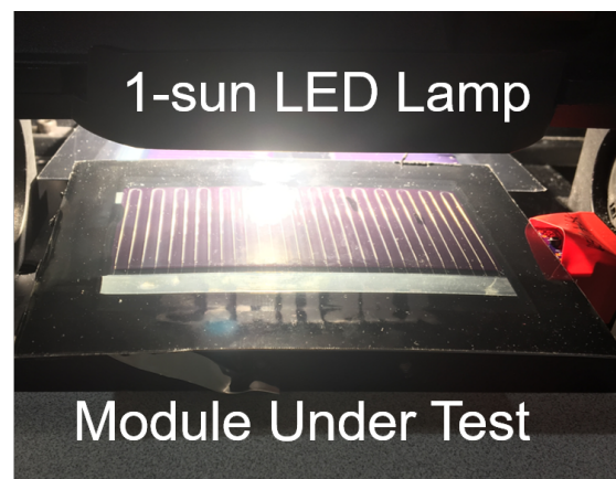
Figure 5.1: Image of the mini-modules studied. The sample is shown during the light soaking procedure used.
