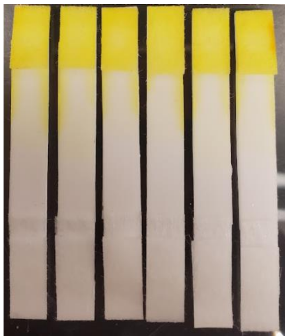
Figure 11: Tested MoReLFA Strips after 10 Minutes of Running Time. Standard Creatinine Concentrations from Left to Right Are 0, 50, 70, 90, 120, 20 \mu\text{M} , Respectively
