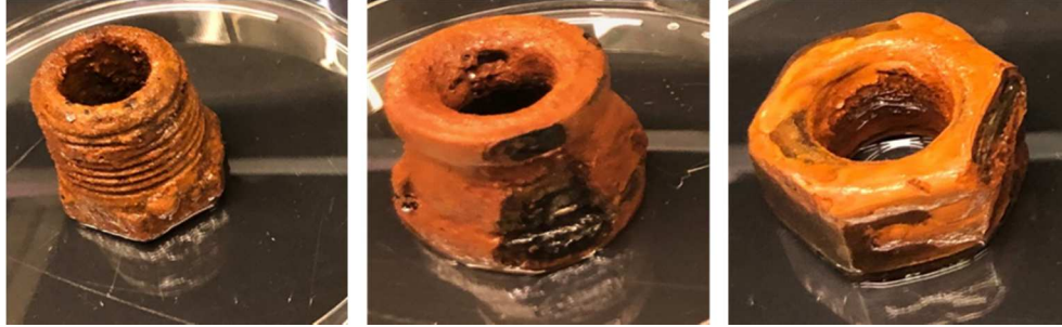
Figure 4. Different shapes of cast iron coupons used in this experiment.
