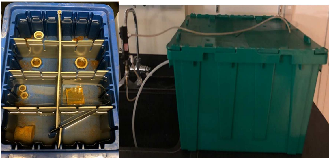
Figure 3. Bioreactor box at Arizona State University-Tempe lab with flow meter, water feed line and discharge line along with individual collection boxes housing various coupons identical to the field bioreactors.
