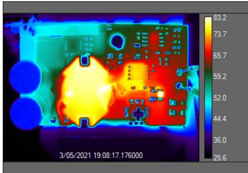
Figure 41 Thermal Image 37 Vin Full Load Top QR Flyback
