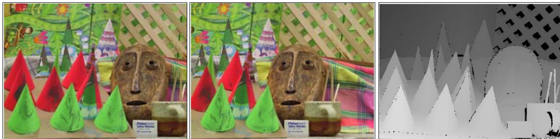
Figure 3.2: Example of Depth Estimation Using Stereo Images, Left Camera Image (Left), Right Camera Image (Center), and Final Disparity Map (Right) (Scharstein, 2003)
