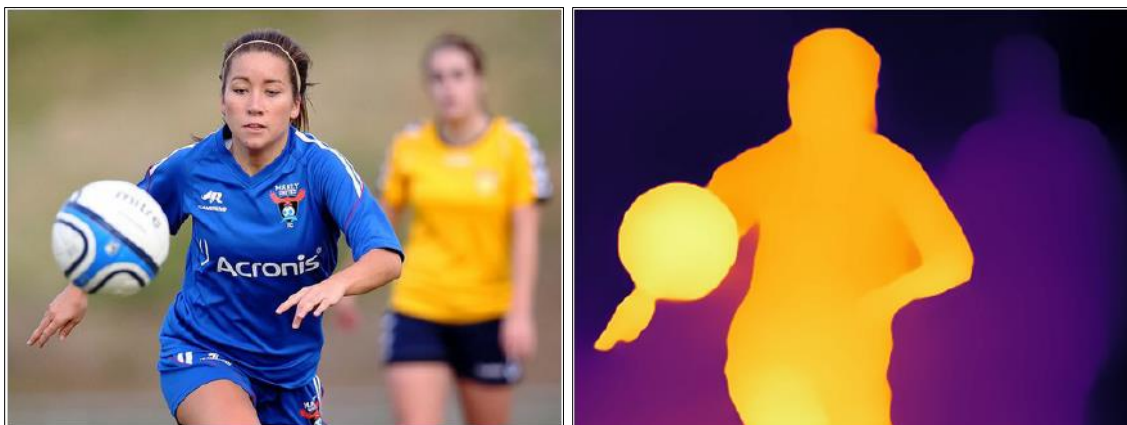
Figure 3.5: Example of Depth Estimation Using Deep Learning (Monocular Cameras), Input Image (Left), Output Image (Right) (Ranftl, 2022)
