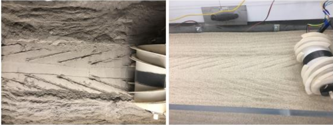
Figure 5. Wake Pattern of Bihelical-Grousered Wheel in BP1 (Left) and Silica Sand (Right)
