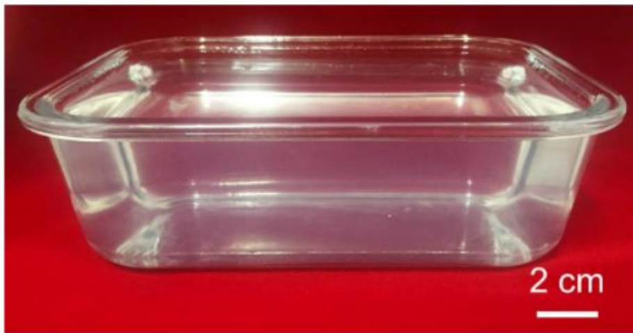
Figure 3-1 The bath is low-cost (<$2/lit), easy and fast to prepare in large quantities, and it is transparent, which facilitates process monitoring.
