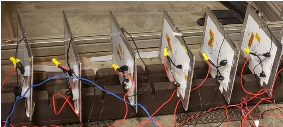
Fig. 30. Test layout for PID in the environmental chamber
