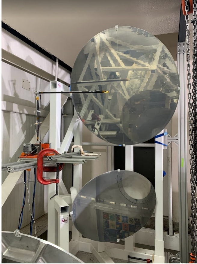
Figure 42. Wyatt robot arm mounted in front of M4. The source on the end of arm is approximately lined up with the center of the mirror.
