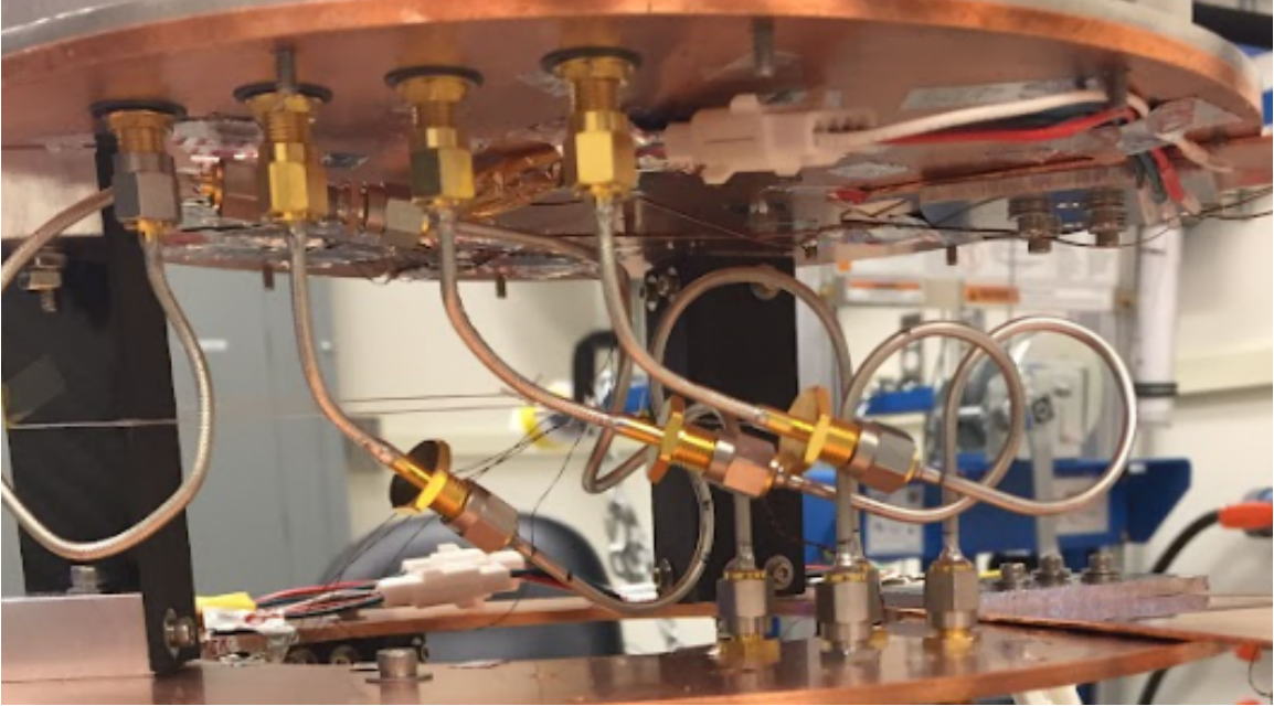
Figure 56. Coax Cables in Baby Beluga.
