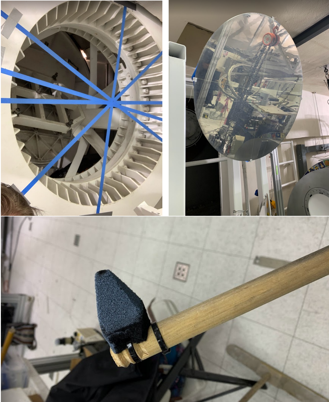
Figure 37. Liquid Nitrogen test set up. Top left shows the tape used to mark the center of the M3 bearing. Top right shows the string used to mark the center of M4. Bottom shows the black body wand used.
