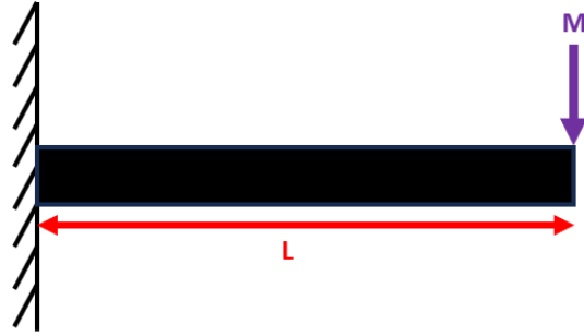
Figure 21. The mirror mount can be simplified as a cantilever beam with a mass concentrated at the end.
