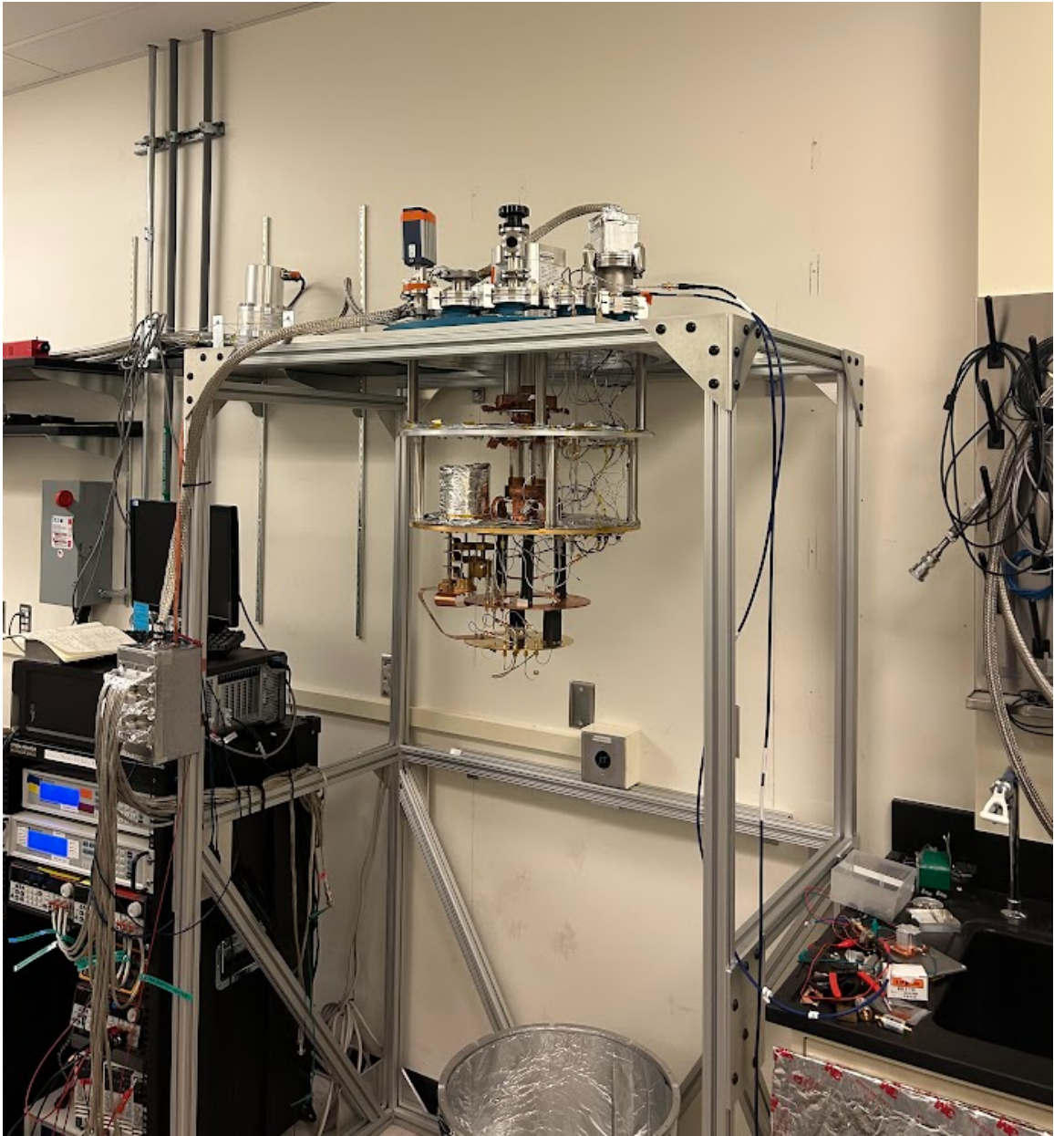
Figure 63. Image of Baby Beluga without its 300 K shell installed on its new mount in the lab.
