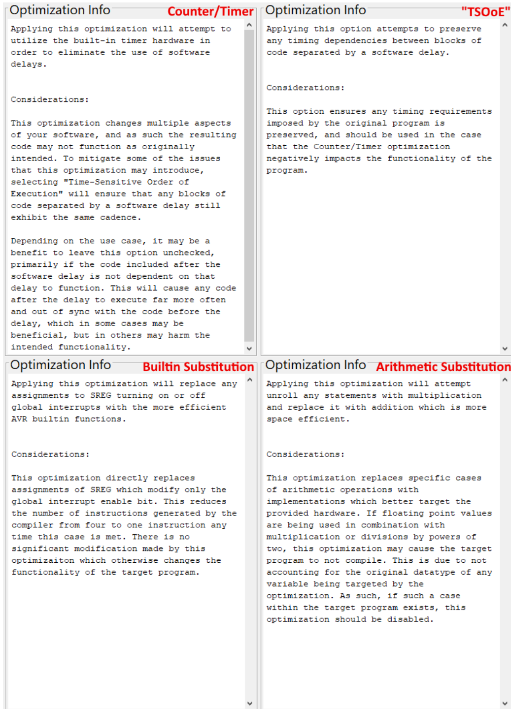
Figure 4.26: The optimization info provided by the Embedded C Source Optimizer for the "Counter/Timer," "Time Sensitive Order of Execution" (or "TSOoE"), "Arithmetic Substitution," and "Built-in Function Substitution" options to aid in the user's understanding of each.
