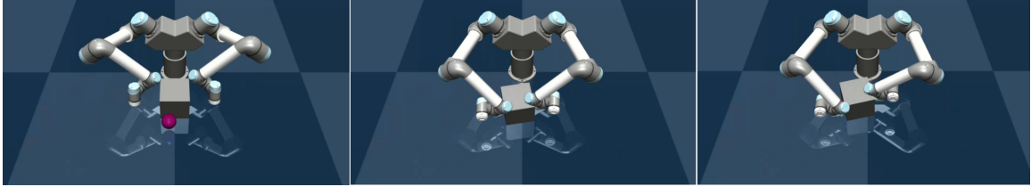
Figure 14. The Box is at the Middle, Close to the Dual UR5 (Test of Training 5000 Times in the First Part of the Experiment)
