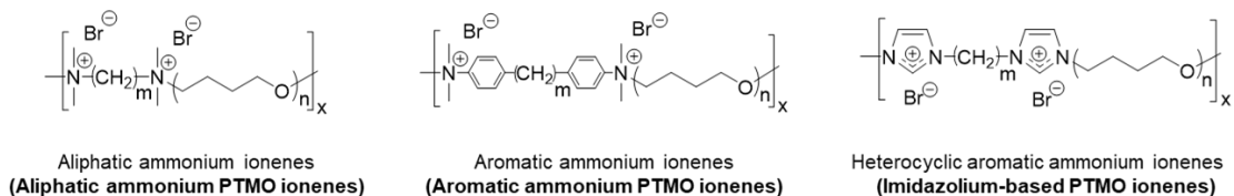
Figure 2.19: Schematic showing the three types of hard segments in segmented ionenes.
