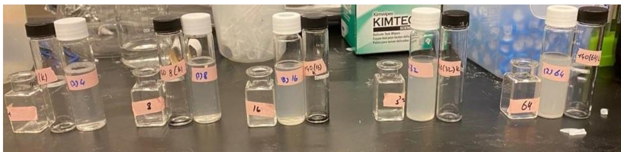
Picture 1. The picture was taken during adsorption testing of GO versus K. The color of the solution changes is proportional to the adsorbate in the solution after completion of the adsorption experiment
