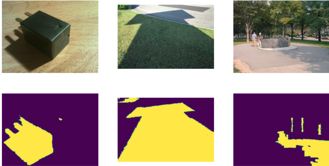
Figure 4.4: Shadow Masks Captured by the Martiny Vision System
