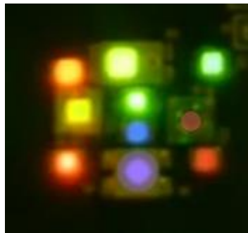
Figure 2.4. Photo of cluster of LEDs with all diodes switched on to give a sense of the actual color output.
