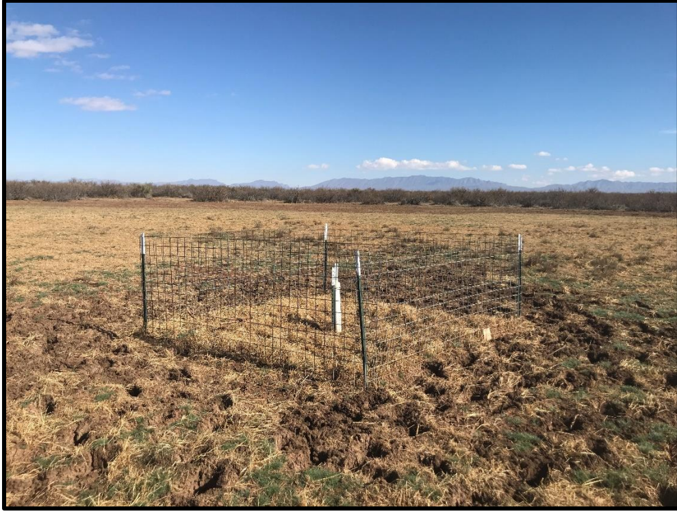
Figure F6. Water level sensor at Playa 6 surrounded by vertisol-like soil trampled by cattle.
