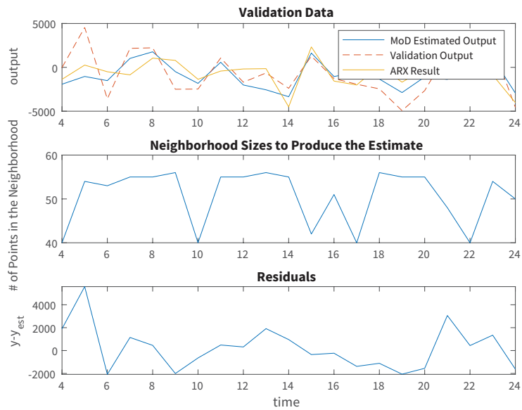
Figure 3.2: Just Walk : MoD and ARX Model Comparison on Validation Data (25% of Participant Data). Output Measured in Steps.
