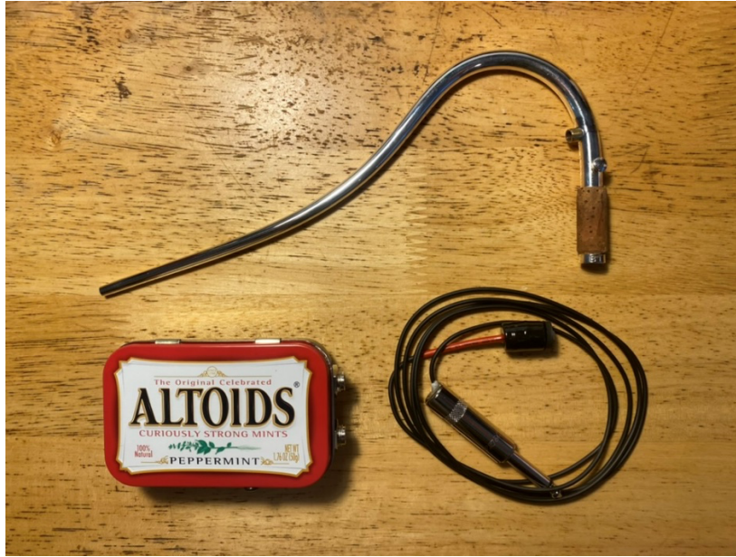
Figure 1: Pickup bocal “Little Jake,” preamp, and screw-in contact microphone
