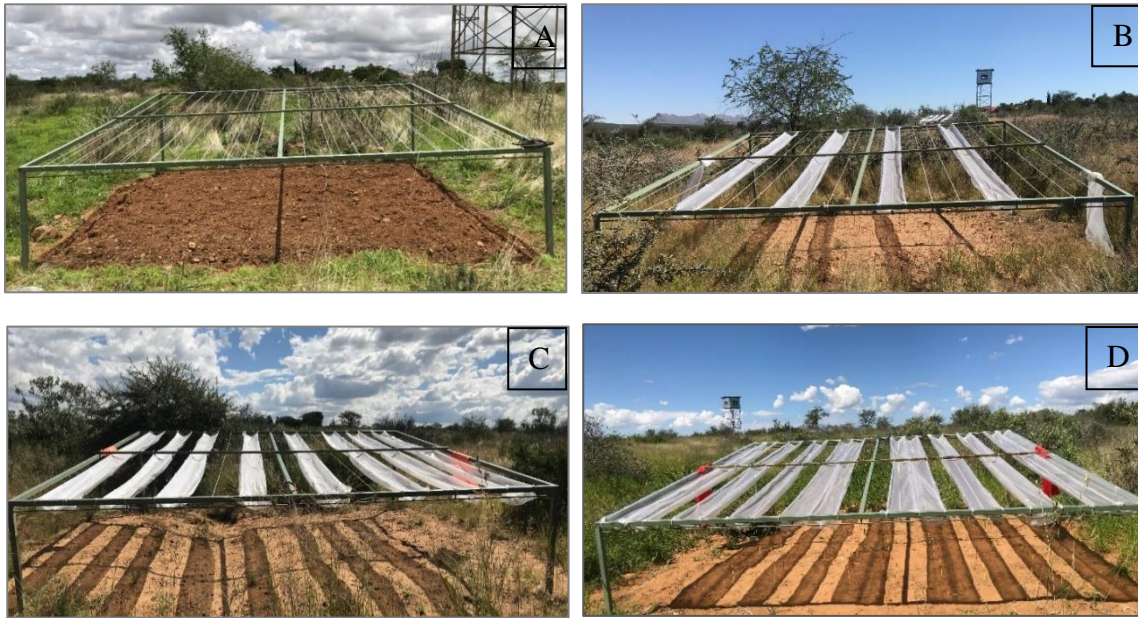
Figure C1. The rainout shelters used in the experiment showing the different treatments. (A) The 0% exclusion plots (representing the control treatment) had no plastic covers. B) The 20% exclusion plots are covered with 4 plastic covers, (C) The 40 % exclusion plots are covered with 8 plastic covers and (D) The 60 % exclusion plots are covered with 12 plastic covers.
