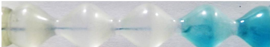
Figure 4. 7. Labels for Transition Onset Location in a Wavy Channel. (a) Label 0: Transition Does Not Occur; (b) Label 1: Transition Occurs from 1st Section; (c) Label 3: Transition Occurs from 3rd Section; (d) Label 4: Transition Occurs from 4th Section.
