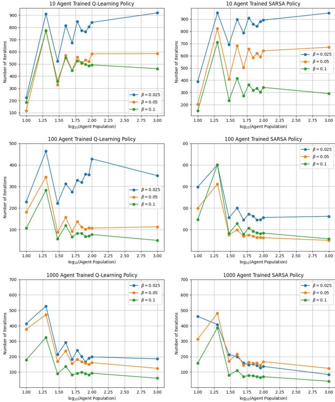
Figure 3.9: Number of iterations until convergence to \hat{S}_{target} versus number of follower agents N (plotted on a log scale) for leader control policies that were trained using Q-Learning ( left column ) and SARSA ( right column ) with D = 10 ; \mu = 0.0025 ; and \beta = 0.025, 0.05 , or 0.1 ; and N = 10, 100 , or 1000 agents. Each circle on the plots marks the mean number of iterations until convergence over 1000 test runs of a leader policy in the simulated grid graph environment in Figure 3.2.
