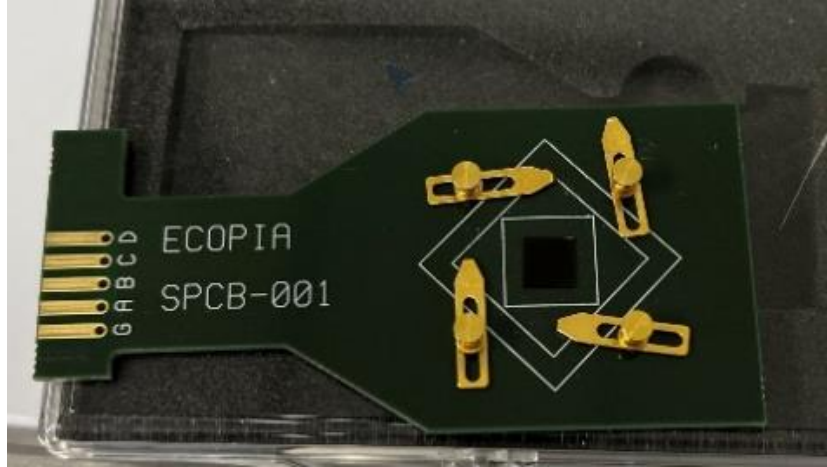
Figure 3.5 Hall Effect Measurement Board. The Contacts Were Placed onto 4 Corners of the Samples and Voltages were Recorded After Injecting Current into the Terminals.
