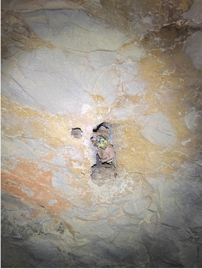
Figure C4. A HOBOT data logger partially concealed in the ceiling of Cave 1 with camouflaged duct tape.
