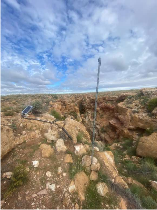
Figure C7. Acoustic monitor set up at Cave 3. Note the solar panel at ground level and microphone attached to a telescoping pole secured in rocks.
