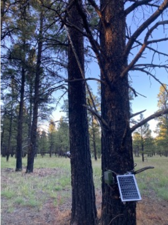
Figure C6. Acoustic monitor set up at Cave 2. Note the solar panel, ARU next to the solar panel, and microphone attached to a telescoping pole in the tree.
