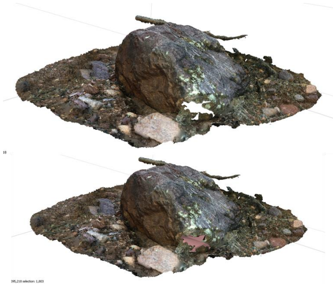
Figure 86- Closing Holes in Mesh.
