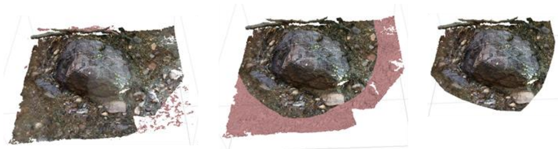
Figure 85- Gradual Selection (right), Manual Selection (middle), and final model boundaries (right).
