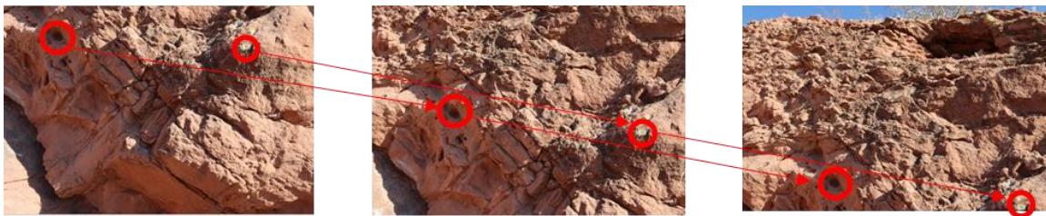
Figure 20- Examples of matching features (red circles) in sequential images. SIFT algorithm used in Metashape SfM to recognize features, align photos, and generate sparse point cloud.
