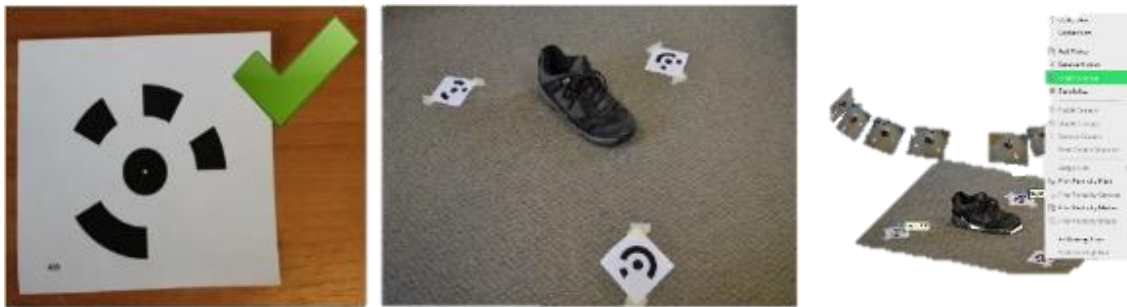
Figure 32- Metashape generated Ground Control Points (GCPs) and their application.
