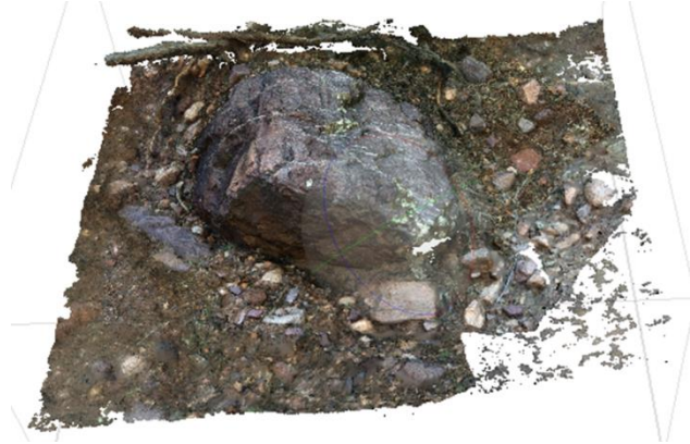
Figure 84- Example of disconnected artifacts (i.e. "shrapnel").
