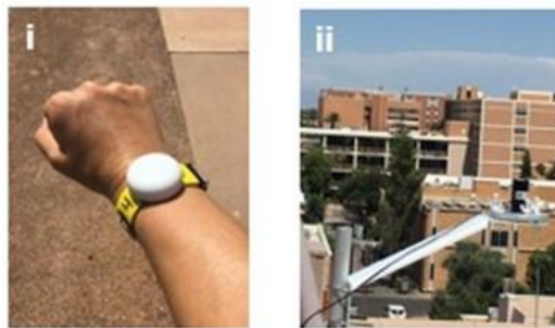
Fig. 3.3: Equipment for measuring UV exposure ratios of personal exposure and ambient UV radiation. (i) wearable dosimeter. 5 (ii) ambient sensor on rooftop for measuring UV in the environment.
