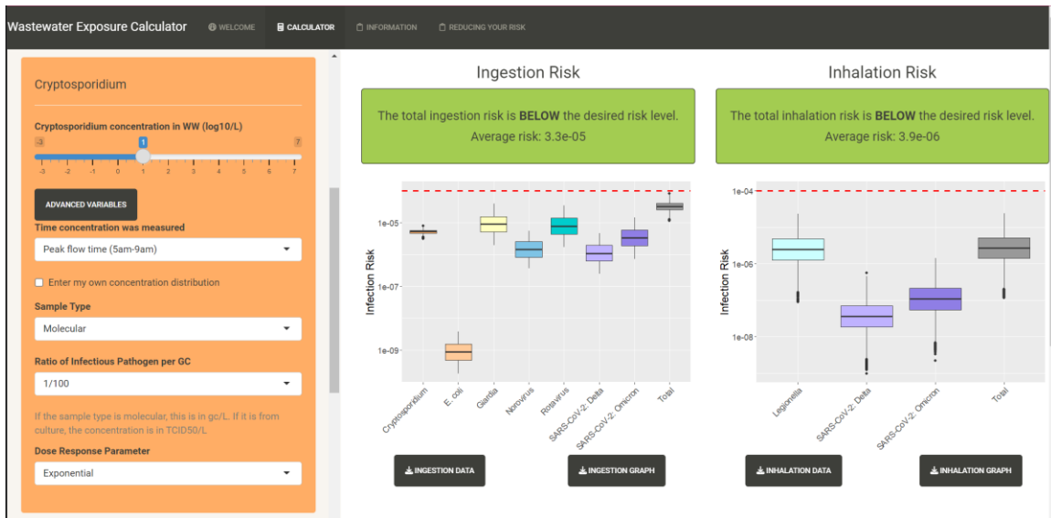
Figure 16: Calculator page with pathogen-specific parameters for C. hominis . Users can enter their concentration of C. hominis in the wastewater and specify the time of day the sample was collected and the sample type, as well as the dose response parameter.
