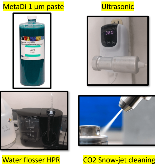
Figure 4.8: Materials were further polished by hand using 1.0 \mu\text{m} MetaDi diamond paste to achieve a pristine mirror surface. The paste was then cleaned off using a 150 PSI water flosser and DI water for 30 minutes per part. All parts were placed in an isopropyl bath and cleaned using a portable ultrasonic device and cleaned for 10 minutes. During assembly in a class 1000 cleanroom the materials were cleaned using a \text{CO}_2 snow-jet gun, ensuring the surfaces were contaminant free before closing the chamber.
