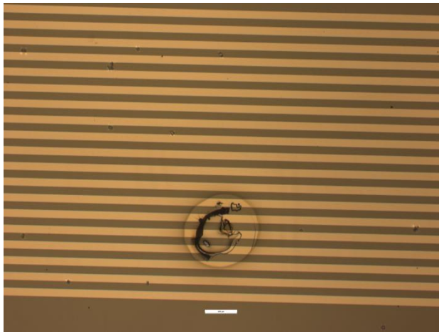
32-45 – Bubble/Hole in tail across u2-u6.
