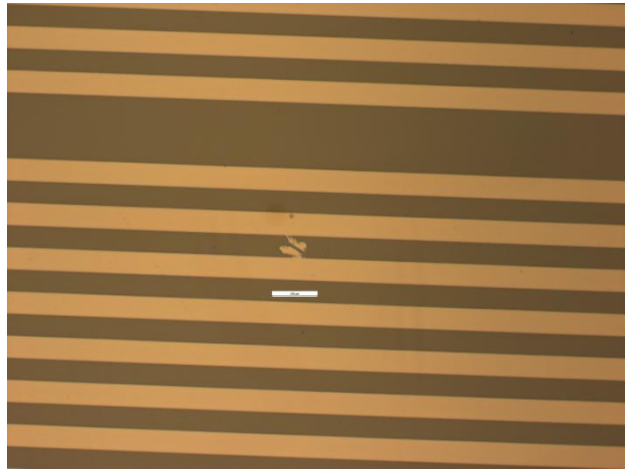
32-46 – Possible short in tail across m16 and GND.
