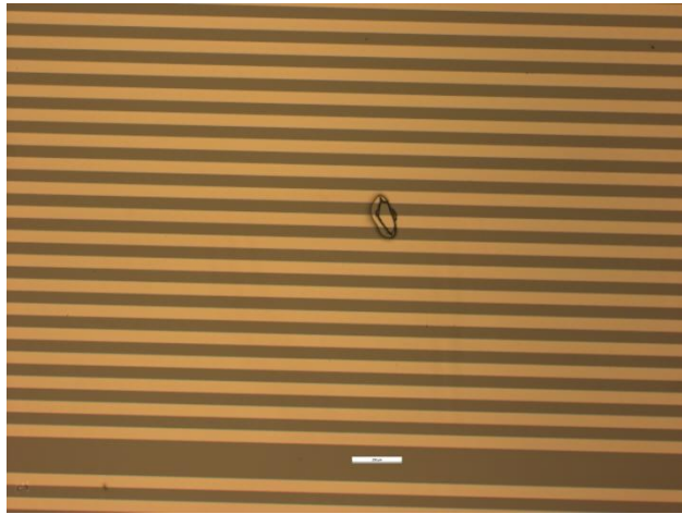
128-4 – Hole in tail of BL section across u23 and u24.
