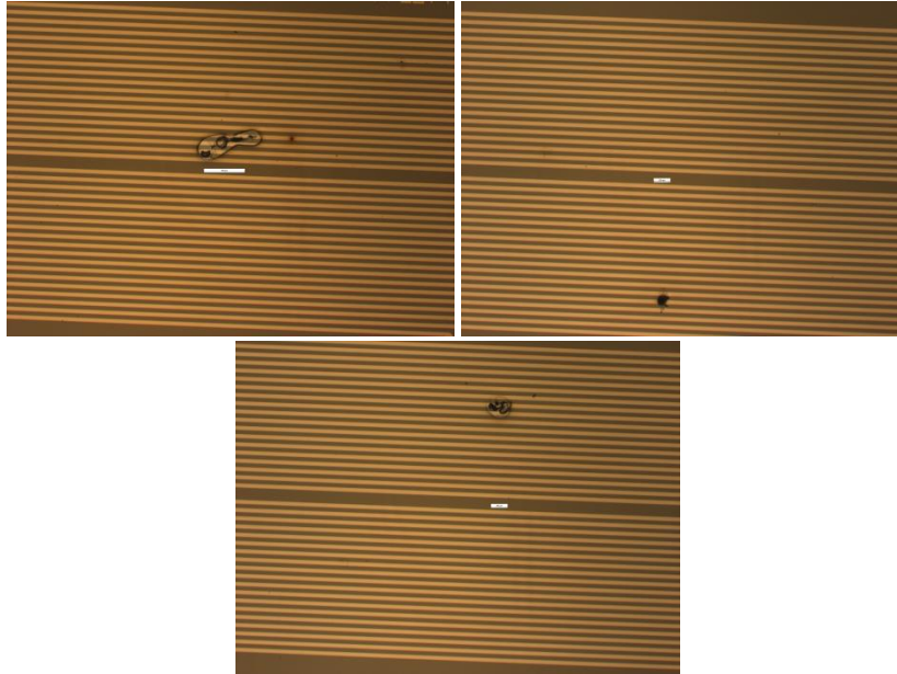
32-52 – (Left) Bubbles/Holes in tail across m32 and u29-u31; (Center) Spot in tail across u4-u5; (Right) Bubbles/Holes in tail across u21-u23.
