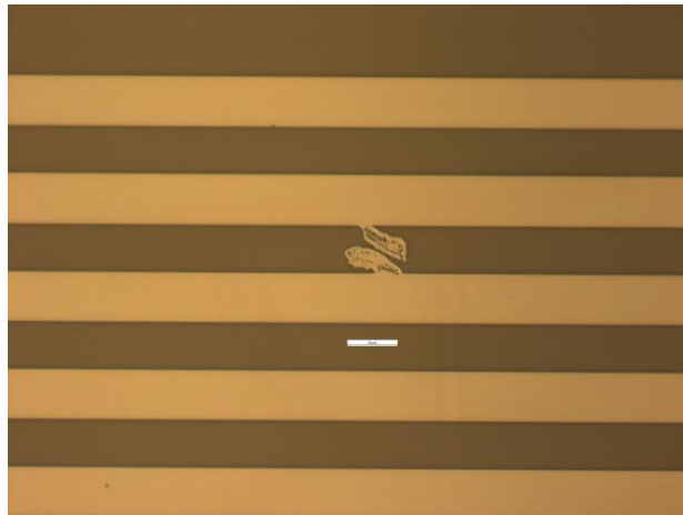
32-58 – Possible short in tail across m16 and GND.
