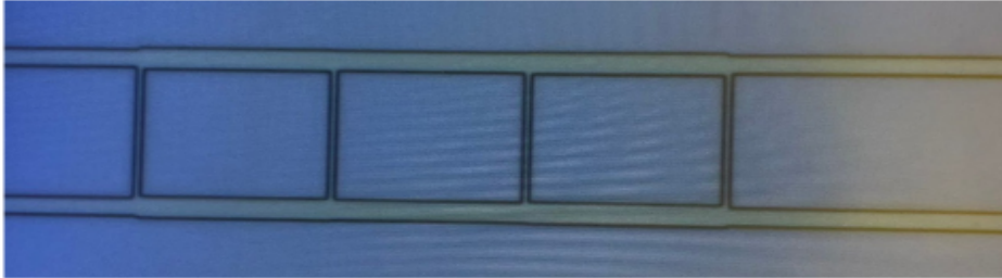
Figure 3.7: The Quadrature Hybrid Coupler After NbN Etch, and SiN Deposition.
