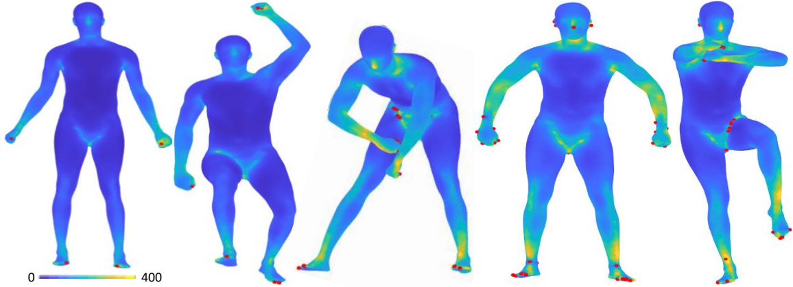
Figure 14. Saliency maps and salient vertices on 3D human models. Salient vertices are marked as red spheres.
