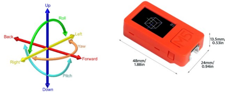
Figure 4.7: Pitch, Yaw, and Roll within a three-dimensional space, parameters generated through M5StickC sensor movement. M5StickC PLUS ESP32-PICO Mini IoT Development Kit.
