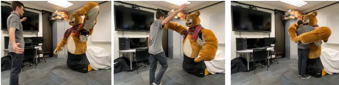
Figure 4. An example of a left-high to right-high interaction. Left: The participant starts with a left-high interaction. Middle: When switching to the right-high hug, the robot responds accordingly. Right: The participant hugs the robot.
