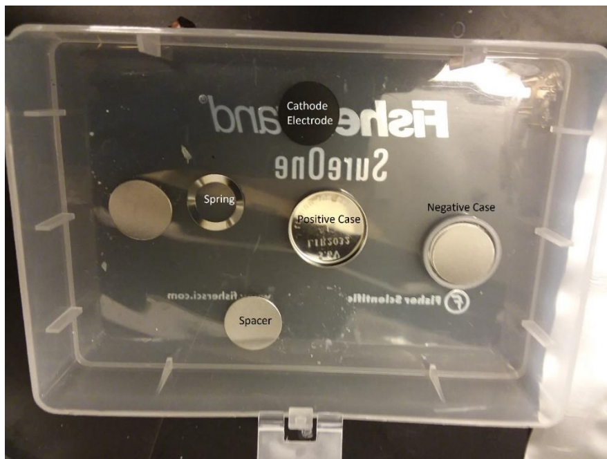
Figure 2.1.1 Labelled parts of a coin cell including the spring, circle electrode, positive case, negative case, and spacers.
