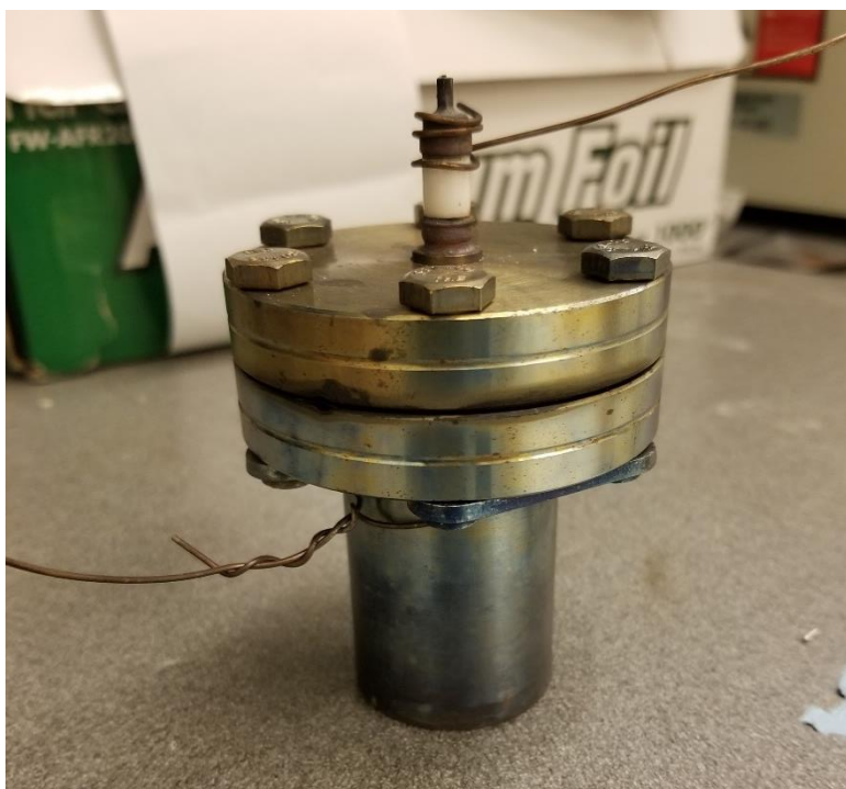
Figure G.1 Photograph of the stainless-steel housing used for the electrochemical cell. The housing consists of a standard 2.75-inch half nipple with the hole on the bottom welded shut with a stainless-steel cap. The top is comprised of a high voltage feedthrough made of stainless steel that is insulated from the flange with alumina. A copper gasket was placed in between the half nipple and feedthrough. The reactions were carried out in a furnace inside an argon glovebox to mitigate the oxidation of the stainless-steel housing at high temperatures.
