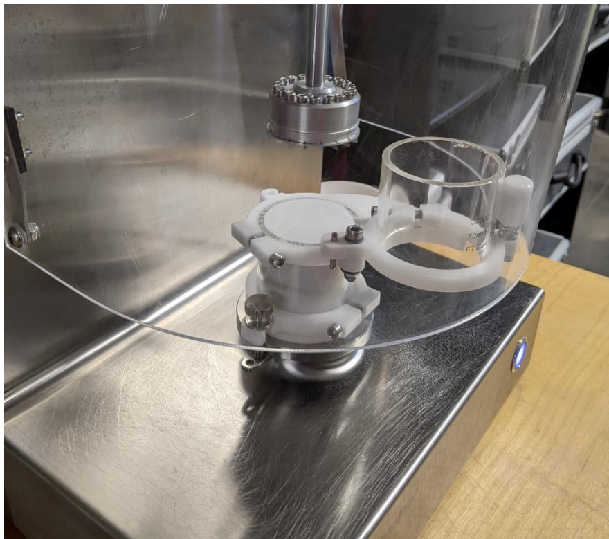
Fig. 2.2 The vessel used for the shear cell test on the FT4. The splitting mechanism is used to get rid of the excess material, resulting in a flat surface for the experiment.
