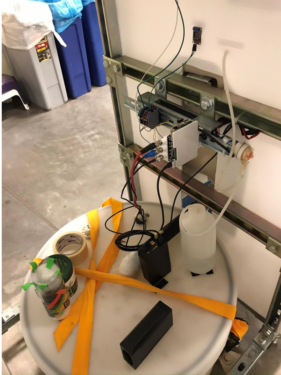
Figure S2. Inside of portable urinal. Sensors are connected to a RaspberryPi that measure pH, conductivity, and temperature of the collected urine. Acetic acid is pumped into the urinal. The tank, capable of holding 25 gallons of urine, is tightly secured down to reduce contamination of urine with microorganisms found in restrooms.
