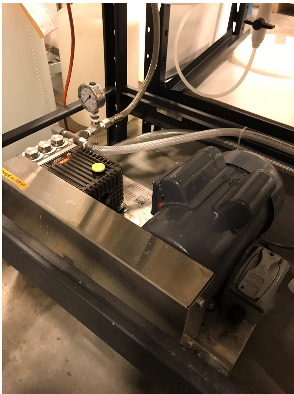
Figure S7. High-pressure pump for system. Feed solution enters from the right, travels through the pump, and exits in the top tube towards the membrane cell.
