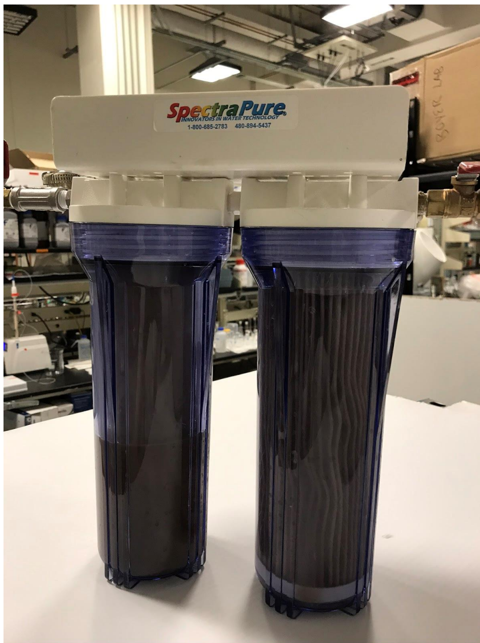
Figure S8. Microfilter system used for microfiltration of real human urine. The left cartridge is a 1- \mu\text{m} sediment filter, and the right cartridge is a 0.2- \mu\text{m} sediment filter.
