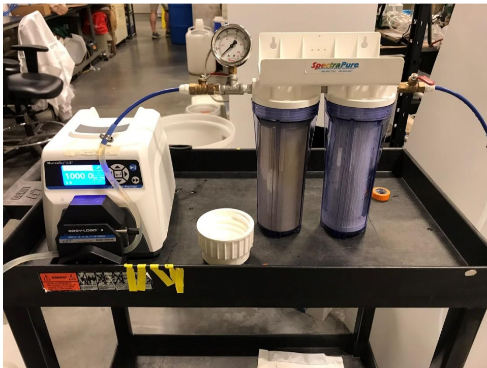
Figure S9. Microfiltration of real human urine. Urine is pumped through a MasterFlex peristaltic pump at 1000 mL/min through the microfilter system at a pressure between 20–60 psi.
