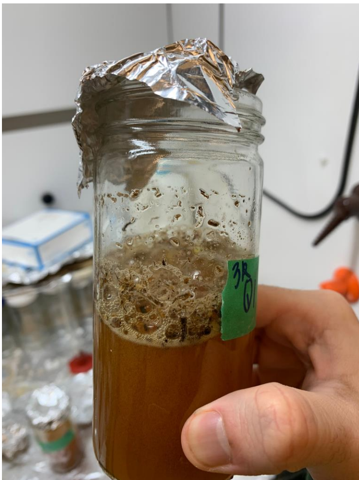
Figure 5. Wet Peroxide Oxidation of soil sample from Q3. Reaction is currently taking place, indicated by presence of bubbles.
