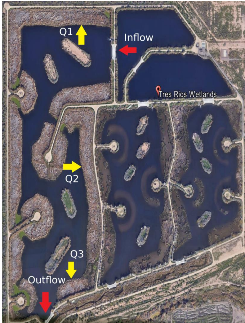
Figure 3. Tres Rios Wetland study site. Red arrows represent inflow (north) and outflow (south). Yellow arrows indicate collection sites for vegetation and soil samples.
