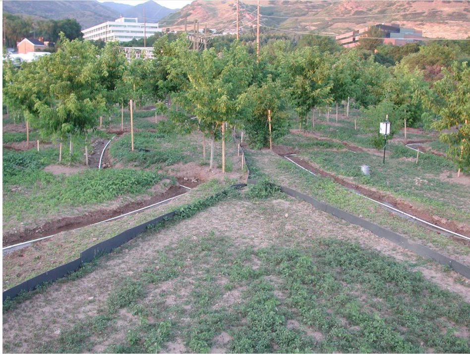
Fig. 1: Artificial stream system at University of Utah common garden that brought free-flowing water within 1 meter of each A. negundo tree. Four channels, approximately 1 m wide and 0.2-0.25 m deep were crafted using a small backhoe in 2005. A 0.75-inch (1.905 cm) diameter PVC pipe was installed along the center of each channel, spanning their entire lengths to supply water. The PVC configuration included a T-junction at the starting point where the streams diverged, and a rejoining point near the endpoint where the streams merged. This design ensured that the garden received water from a single irrigation source. Water was dispensed from the PVC piping into the channels through 360° adjustable bubblers. The drainage system comprised two 50-liter catch basins that emptied into a large lowland area near Red Butte Creek.
