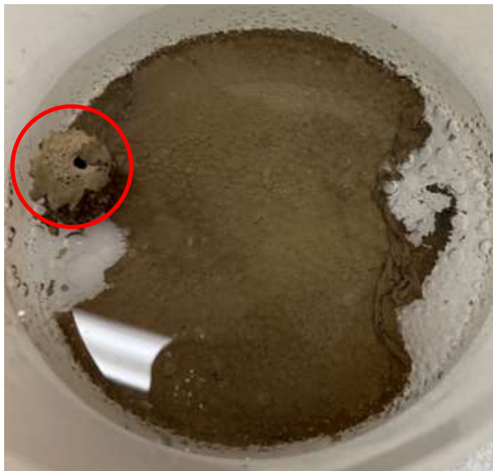
Figure 3-9: Electrowon Silver from Solar Cells with the Silver Located Around the WE and the Bottom
